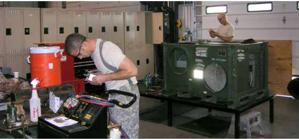
Two Soldiers recharge an environmental control unit as part of their hands-on training at the National Maintenance Training Center at Camp Dodge, Iowa.
